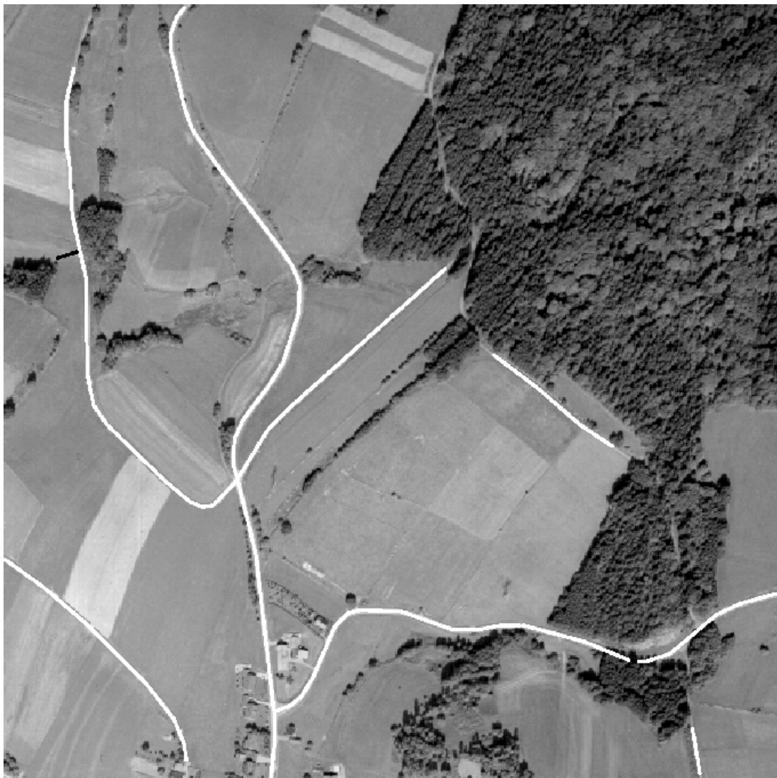
Figure 1: Result of automatic road extraction for image “Marchetsreut” using the TUM approach (white lines: correct result; black lines: incorrect result, i.e., not matched to ground truth).
