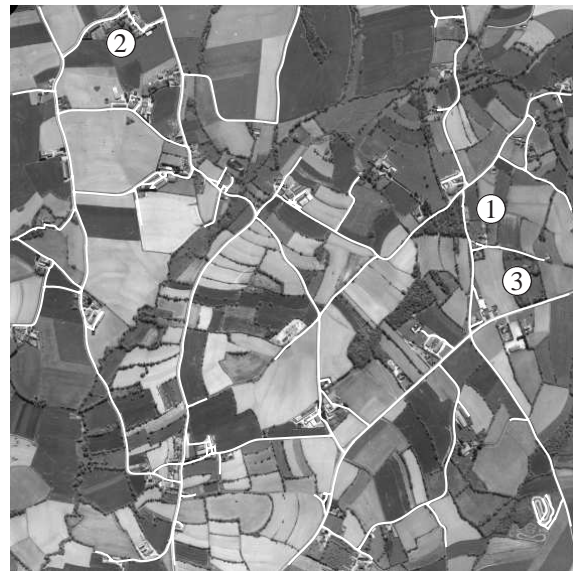
Figure 18: Result of the completion of the extracted road network; the numbers refer to Fig. 19
