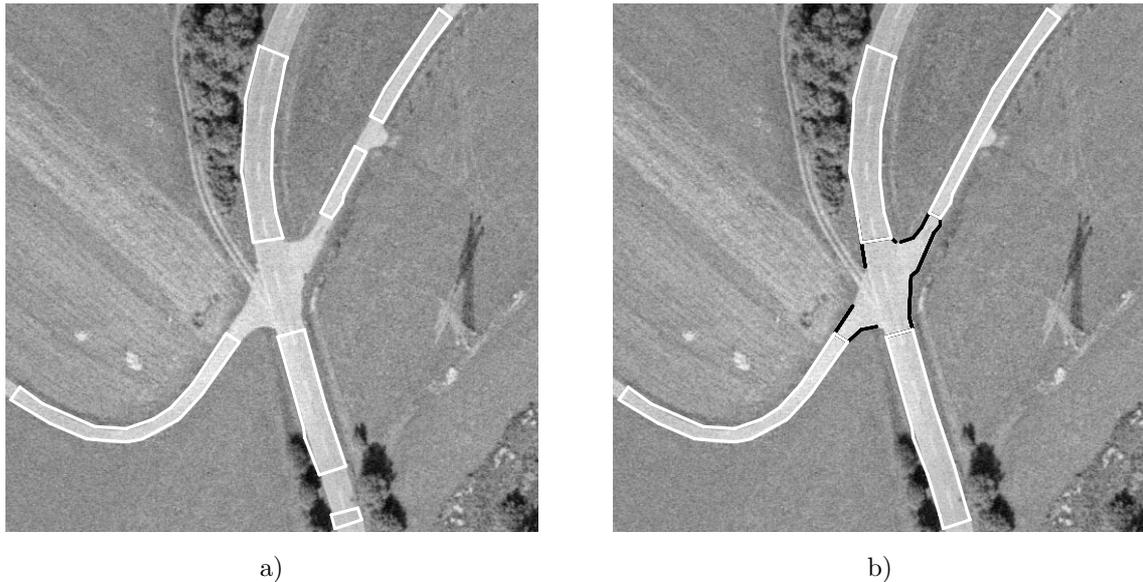
**Figure 14.** a) Road-segments after closing gaps of first-kind b) Road-segments after closing gaps of second-kind (white), Intersection polygons (black)
