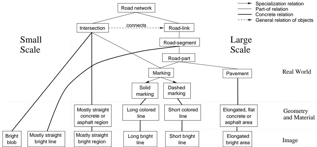
Figure 1. Road model: different resolutions and points of view
