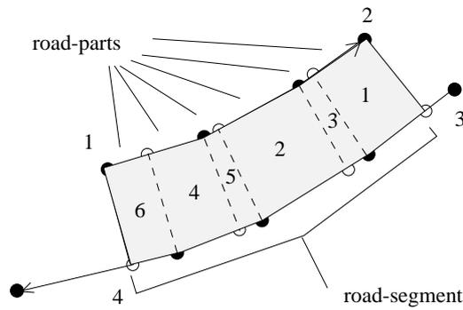
Figure 8. Construction of road-parts and road-segment
