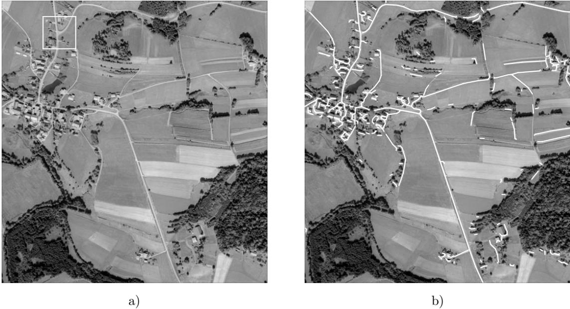
**Figure 6.** a) Image at low resolution. b) Hypotheses for road axes at low resolution.
