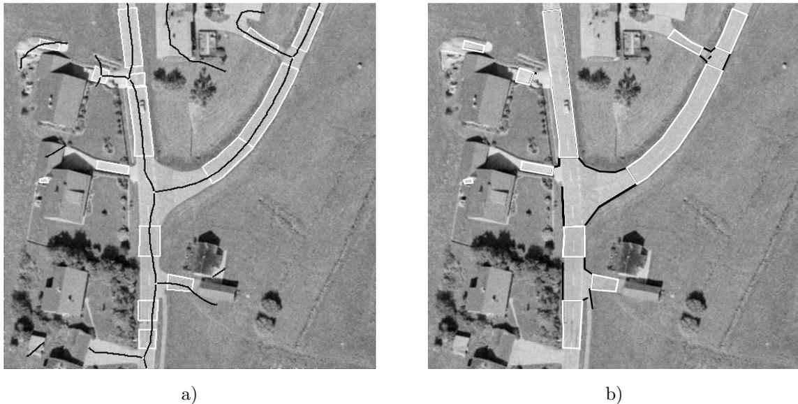
**Figure 11.** a) Road-segments (white), lines (black) and junctions (white points). b) Polygons of intersection areas (black) and road-segments (white), after closing of small gaps.
