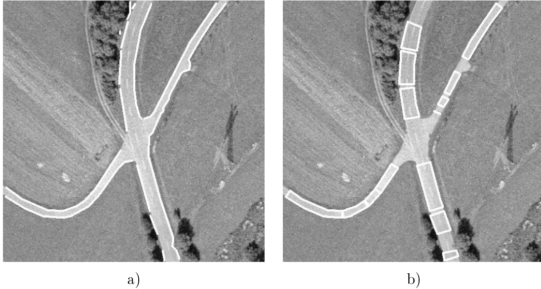
Fig. 11: a) Roadsides b) Road-segments
