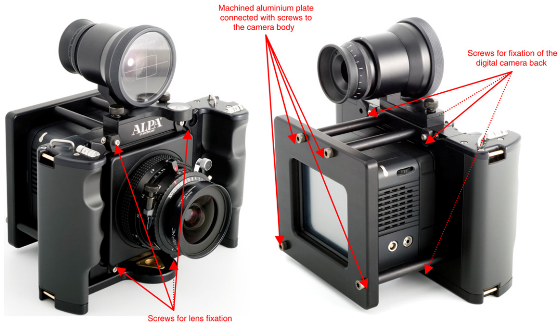
Fig. 1. Alpa 12 WA with the digital back and the lens fixed to the camera with screws. Four clamps in the front and four clamps in the back of the standard camera were replaced with screws. In addition to that, an aluminium plate was connected with screws to the camera providing extra support for the digital back.
