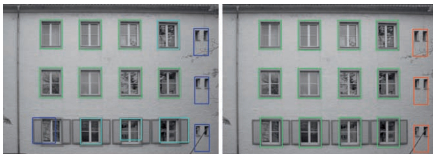
Fig. 6: Validation of hypotheses – left: Before verification. Hypotheses with grade 5 as green, with grade 4 as yellow, with grade 3 as cyan, and with grade 2 as blue rectangles; right: After verification: green – accepted, red – rejected hypotheses.
