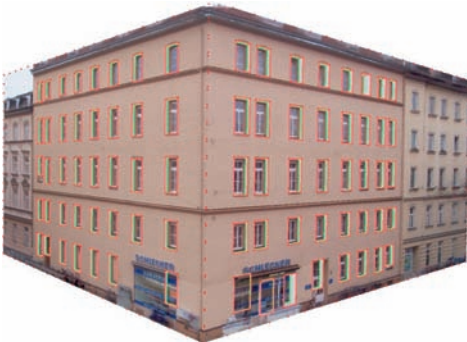
Fig. 13: Result for sequence Bordeaux Square with individual windows constructed from eleven images – explanation cf. Fig. 12.
