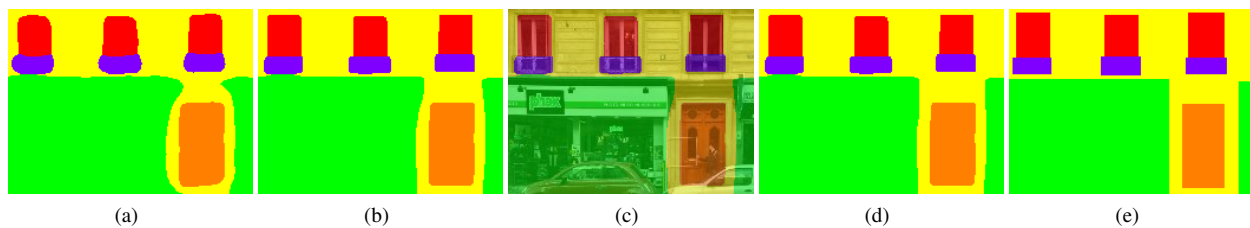
Figure 5. Iterative delineation. Image (a) results from the Structured Random Forest. (b) gives results after 10 iterations, (c) results after 10 iterations mapped into the input image, (d) results after 50 iterations and (e) ground truth. One can observe that the object delineation is very accurate even after only the 10th iterations. Colors see Fig. 2.
