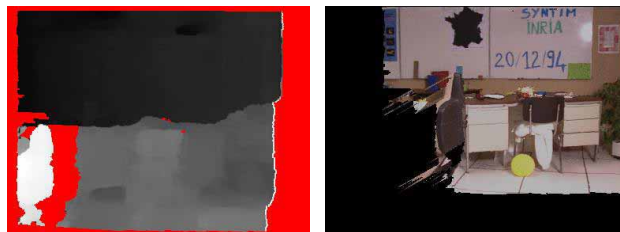
Figure 12: Result (occluded regions in red / light gray) with the same parameters as in Table 3 (left) and visualization (occluded regions in black) with trifocal tensor according to (Avidan and Shashua, 1998) (right)
