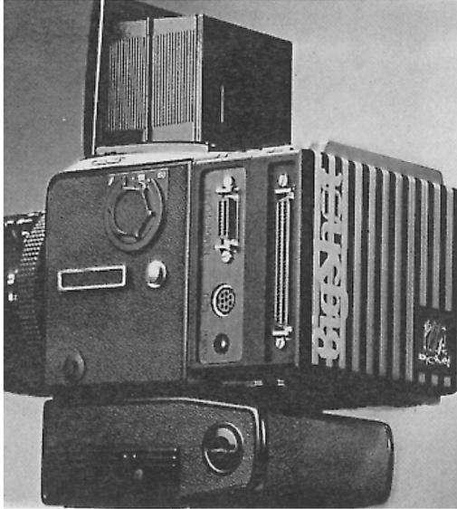
FIG. 1. Dicomed BigShot digital camera back attached to a Hasselblad camera body.
