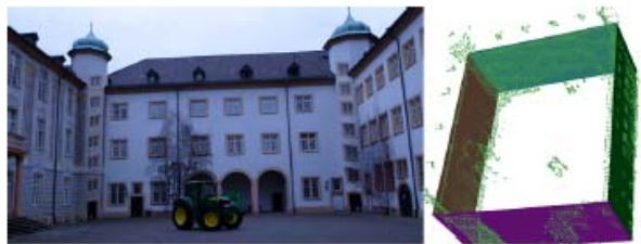
Figure 12: Left: Image of the inner yard of a building consisting of four major walls with many ornaments and two cylindrical towers in the yard's corners. Right: The derived point cloud consists of 1 million points, the four major walls were successfully detected, segmented and connected.
