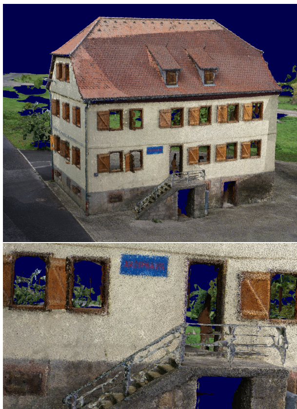
Figure 3. Reconstructed dense point cloud with surface mesh containing more than 25 million 3D points and more than 50 million triangles. This result is not the highest resolution we can obtain, but we are still able to visualise this model. The lower part shows a close view, where details as the sign left of the door or the handrails of the stairs can be recognized.
