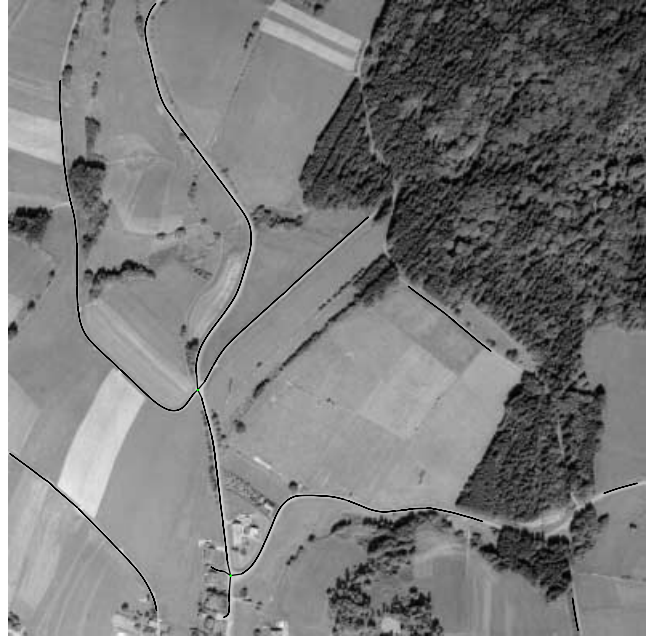
Fig. 13. Road extraction in image “Marchetsreut” (centerlines only)
