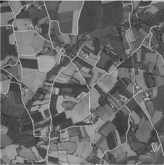
Fig. 12. Road extraction in image “Erquy” (centerlines only)
