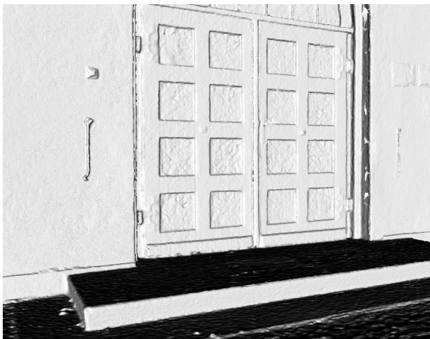
Figure 5: Dense 3D reconstruction of a small part of the scene shown in Fig. 4
