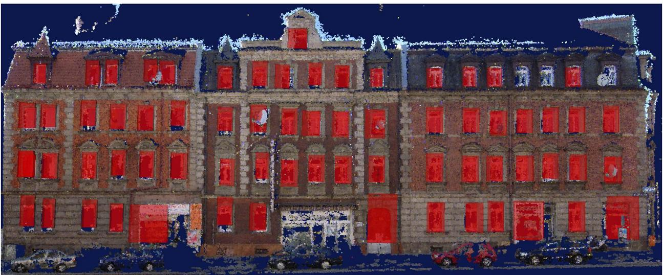
Figure 6: Dense point cloud of several façades with windows and doors marked by red boxes.
