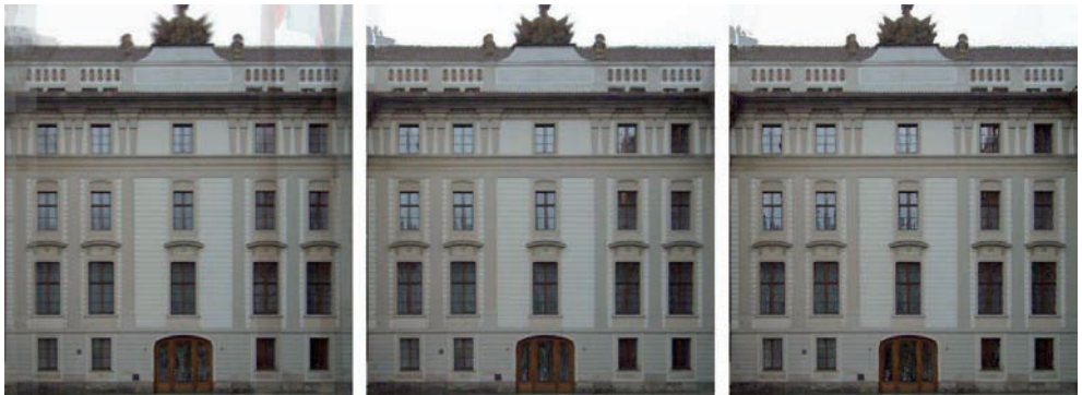
Fig. 4: Facade image derived from the six images given in Fig. 1 – left: average; center: median; right: consensus.
