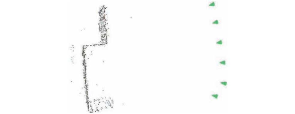
Fig. 2: 3D points, colored according to the pixels, and cameras (green pyramids, the tip symbolizing the projection center and the base giving the direction of the camera) derived from the images given in Fig. 1.
