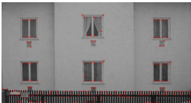
Figure 3. Facade (left) and evidence for window centers (yellow dots, right) both with Förstner points (red crosses)
