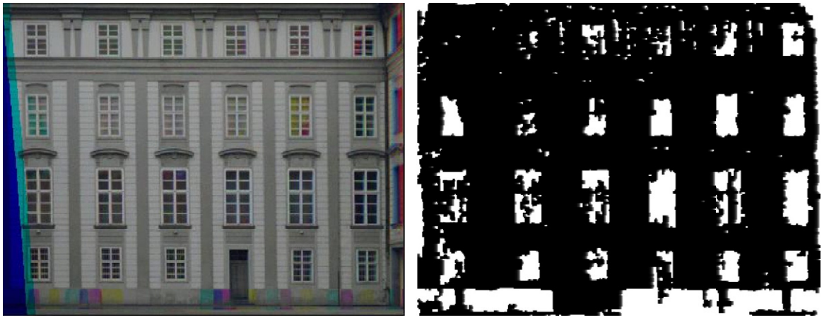
Fig. 3. Three black-and-white images projected onto one of the facade planes mapped into the red, green, and blue image channel showing radiometric differences, but also deviations from the plane (left) and pixels on the plane (black), i.e., pixels not classified as outliers (right).
