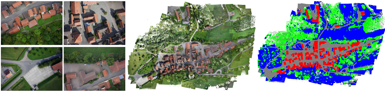
Figure 1. Village dataset: The four images on the left each show one of 296 36-megapixel input images acquired from an Unmanned Aerial Vehicle (UAV). In the middle the noisy point cloud derived from disparity maps accumulating half a billion 3D points is given. On the right the classification results for buildings (red), ground (gray), grass (blue) and trees (green) are presented. In spite of the huge amount of input data, our method allows for the classification within a couple of hours on a single PC.
