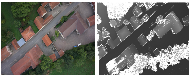
Figure 2. Example image of the urban dataset (Figure 1) and the corresponding disparity map from SGM considering twelve overlapping images showing partly the same scene. The white areas represent areas filtered by consistency checks in SGM.
