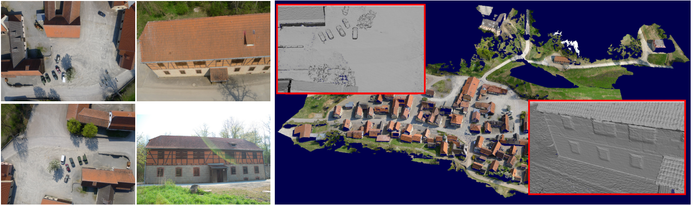
Fig. 10: Left: four sample images of a registered image set of 822 high-resolution images. Right: The complete textured reconstructed model, as well as zoomed views rendered without texture to visualize the preservation of small details. Despite the space division strategy, the 3D model has seamless and consistent surfaces.
