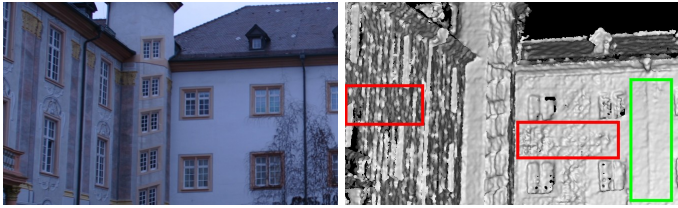
Fig. 4: Varying disparity quality. Left: Zoomed region of an input image of the Ettligen30 sequence (Strecha et al., 2008). Right: Surface orientation derived from the disparity map computed by SGM visualized using a linear coding from 0^\circ (light) to 90^\circ (dark). The surface orientation gives a good impression of the reconstruction quality. Accuracy is lower in slanted and untextured regions (left and center red box), and higher in textured fronto-parallel regions (right green box).
