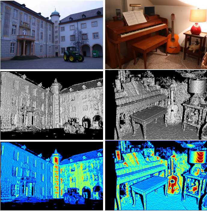
Fig. 6: Visualization of computed TV classes for each pixel. Top: Input images. Middle: Disparity surface orientation (as in Fig. 4) providing an impression of the local reconstruction quality. Bottom: TV classes measuring disparity smoothness, ranging from 1 (blue) to 20 (red). Fronto-parallel textured surfaces lead to higher class numbers.
