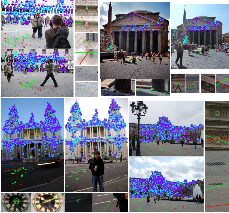
Fig. 6. Four examples for optimized essential matrices from image pairs. Because of challenging texture, perspective, resolution and lighting conditions in these examples MODS is used for ground-point matching. Verified features are color-coded as in Fig. 5. The zoomed images show examples for ground and non-ground matches. While the non-ground matches are correct for both methods, the ground points were only related correctly with our method (green epipolar line). The red epipolar line, representing the five-point essential matrix, shows an error of tens of pixels for ground images.
