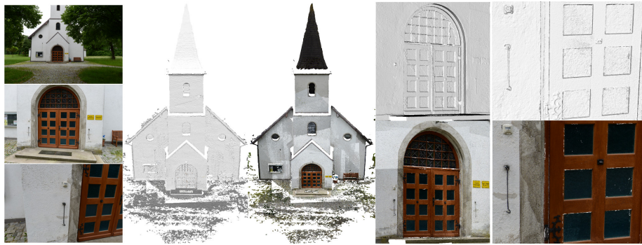
Fig. 2. Textured and shaded multi-resolution 3D model from 54 images (left column). The size of the largest voxels is about 200 times larger than the size of the smallest.
