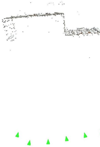
Figure 2. 3D points (red) and cameras (green pyramids, the tip symbolizing the projection center and the base giving the direction of the camera) derived from the images given in Figure 1
