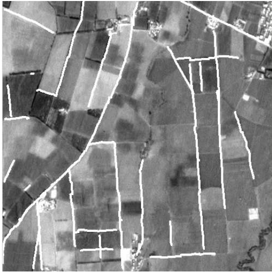
Figure 7: Result of road extraction in agricultural area
