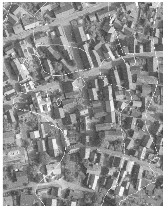
Figure 12: Contour lines derived from DTM after filtering and smoothing (built-up area)
