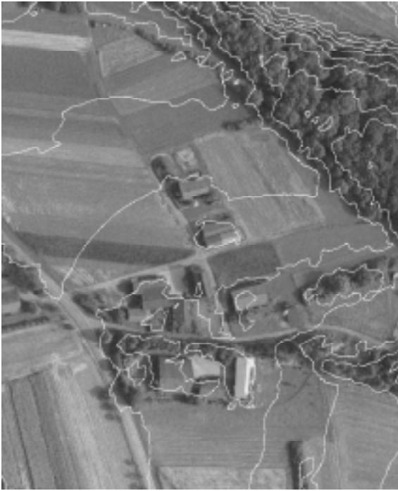
Figure 9: Contour lines derived from DTM without filtering and smoothing
