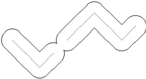
Figure 5: Buffer resulting from conventional dilation using a circle as structuring element.
