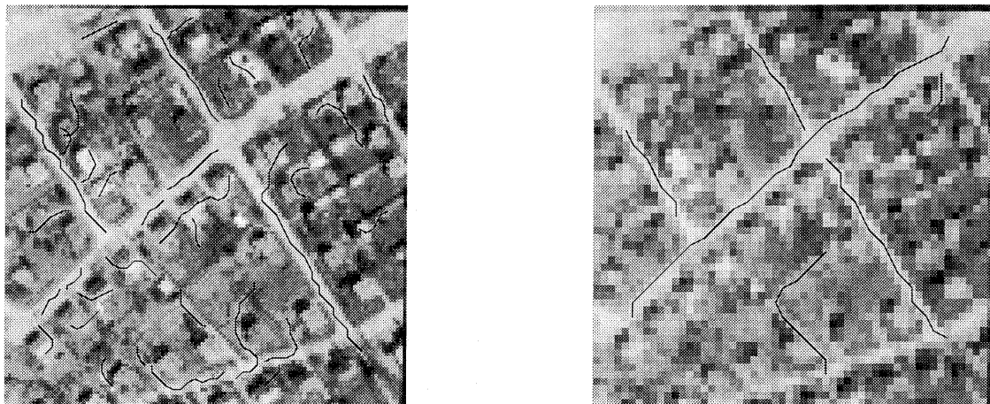
Figure 7: Detection of bright lines — a) (left) Larger scale, b) (right) Small scale
