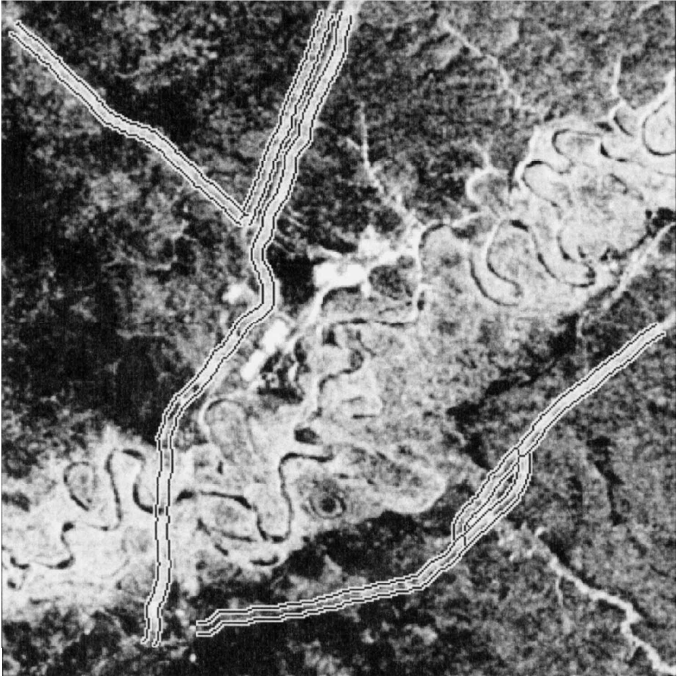
Figure 9. Pipelines and railroads extracted with ziplock snakes from posterior odds superimposed on the SAR magnitude image. The geographic location of the site can be taken from figure 11.
