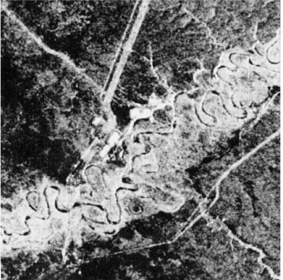
Figure 4. Multitemporal histogram-equalized magnitude (square root of intensity) of an ERS-SAR scene. Approximate scale of the figure is 1:130 000, the size of the area is 17 \times 17 \text{ km}^2 . The geographic location of the site can be taken from figure 11.
