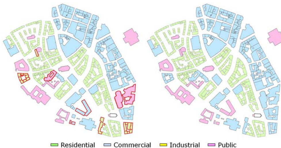
Figure 7. Example data (cadastral map) of Hanover, Germany: the labeling result (left) and the ground truth (right). The incorrectly labeled buildings are highlighted with bold red contours in the result.
