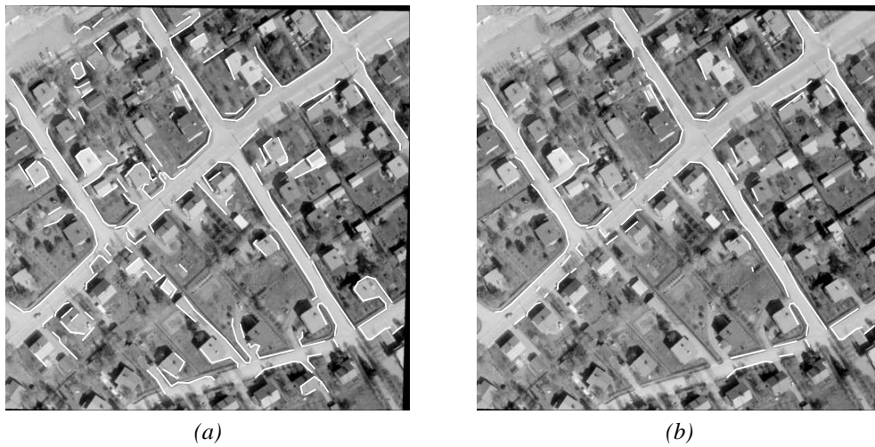
Figure 10: Bright elongated regions in large scale (a) and result of fusing lines in small scale and bright elongated regions in large scale (b)
