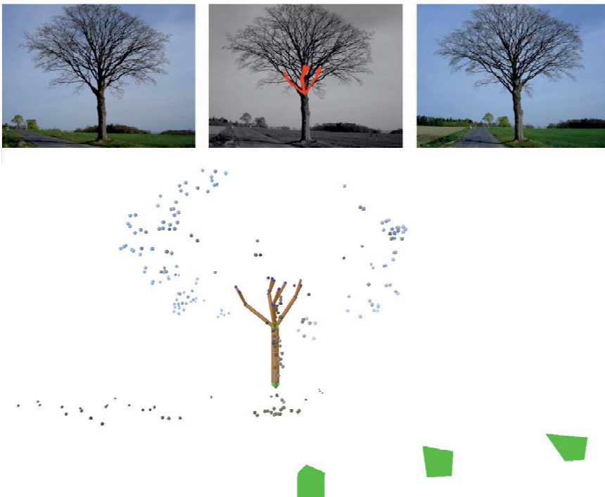
Fig. 5: Result for an image triplet limited to the trunk and the first two levels of branches – branches projected into images (top) as well as the 3D tree, the cameras as (green) pyramids, and points used by the orientation procedure (bottom).
