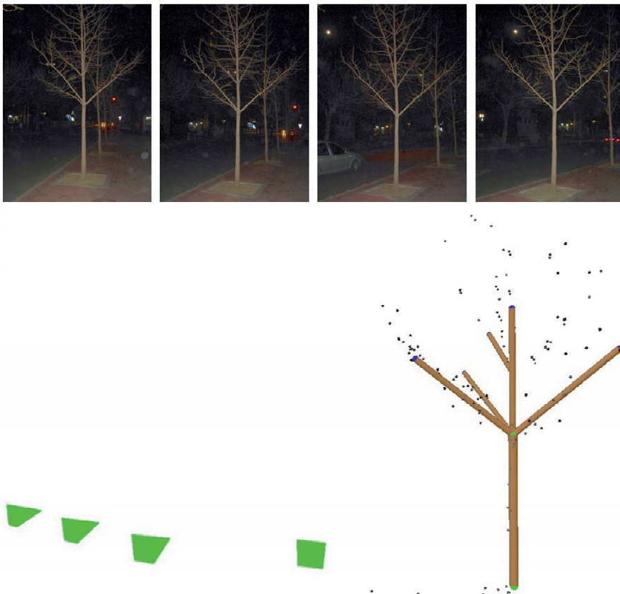
Fig. 4: Result for a Chinese image quadruple limited to the trunk and the first two levels of branches – Images (top) as well as the 3D tree, the cameras as (green) pyramids, and points used by the orientation procedure (bottom).
