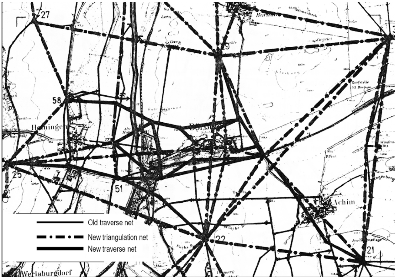
Figure V-4. Control Networks in Börbum area.
