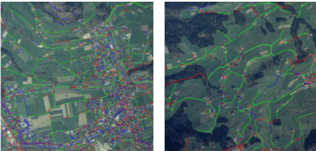
**Figure 1: Aerial1 – Zhang (left), Aerial2 – Gerke\_WB (right); correctly extracted roads are given in green, incorrectly extracted roads in blue, and red marks the part of the ground truth for roads which could not be extracted.**
