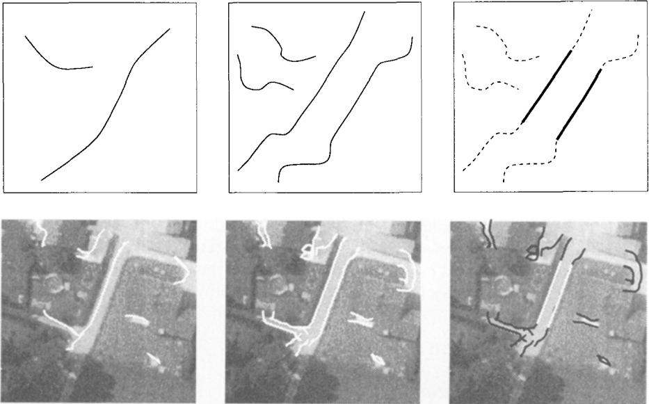
**Fig. 2.** Extraction of *salient* roads. (a) Extraction of lines (b) Optimization of ribbons' boundaries (c) Selection of ribbons' parts with constant width. Only the white ribbon is accepted as a correct hypothesis for a *salient* road.
