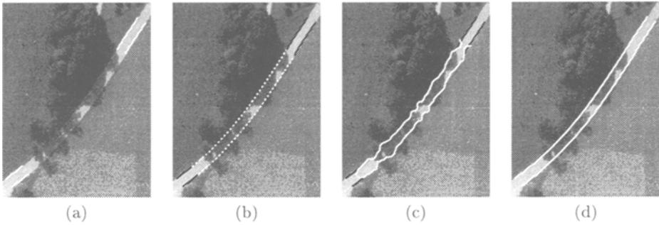
**Fig. 3.** Extraction of *non-salient* roads. (a) Selection of initial hypothesis (b) Extraction of optimal path; (c) Verification by optimization of width (d) Selection of hypothesis with constant width
