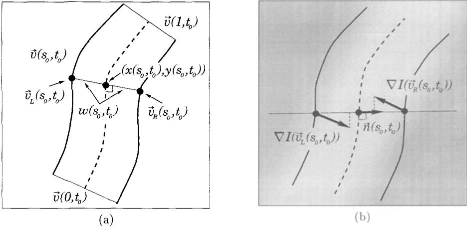
**Fig. 1.** (a) Parametric representation of the ribbon snake. Each slice of the ribbon  $\mathbf{v}(s_0, t_0)$  is characterized by its center  $(x(s_0, t_0), y(s_0, t_0))$  and width  $w(s_0, t_0)$ . Center and width define points  $\mathbf{v}_L(s_0, t_0)$  and  $\mathbf{v}_R(s_0, t_0)$  corresponding to the left and right side of the ribbon. (b) Image gradients for the left and the right side and their projection to the ribbon's unit normal vector  $\mathbf{n}(s_0, t_0)$ .
