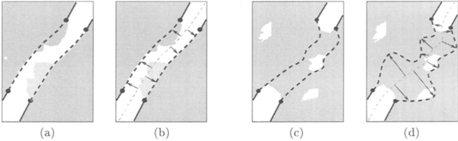
**Fig. 5.** Verification of hypotheses by expanding the width (a),(b) Verification of correct hypothesis. Since the ribbon's centerline in (b) is fixed, the contrast at only one side is enough to stop the expansion (c),(d) Verification of wrong hypothesis. Random features result in a big variation of the width (d).
