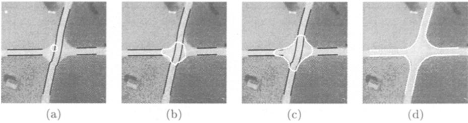
**Fig. 7.** Steps of the optimization of a crossing's outline (a) Initial state of the closed snake (b),(c) 10th and 20th step (d) Final result.
