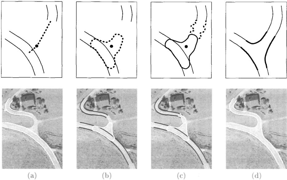
**Fig. 6.** Extraction of crossings (a) Selection of initial hypothesis (b) Approximation of the crossing's outline (c) Verification of connections to adjacent roads (d) Construction and connection of the crossing
