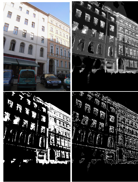
Figure 9. From top left to bottom right: façade image, visualization of colour differences to complete sequence, segmentation of colour difference image using the 0.7 quantile of pixels unequal 0, image with gradient magnitudes.
