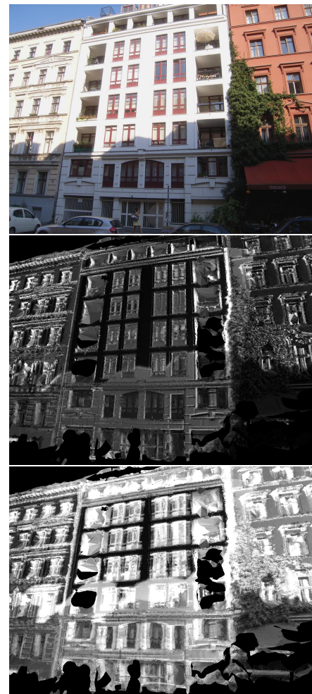
Figure 5. From top to bottom: façade image, visualization of colour differences to neighbouring images only, and visualization of colour differences to complete sequence. The façade in the center of the image reflects with a very bright intensity. If compared to the neighbouring images only, the differences are very small. Consequently, the wall diffusely reflects the light. If the colour differences are calculated over the complete sequence, the borders between wall and windows do not stay so clear. This might be caused by a specular fraction of the reflection or by incorrect reconstructed object surfaces in the mesh close to the window openings.
