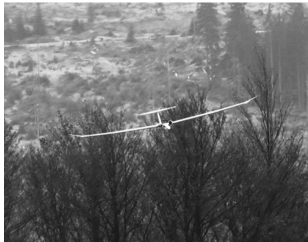
Fig. 1: Data acquisition at a test site in the Bavarian Forest National Park. Left: Preparing the UAV for its flight using a FPV flight guidance system. Right: UAV during its flight. Rough start and landing conditions as visible in the background can get avoided by using UAV platforms with hand launch and net landing capabilities as the shown power glider.
