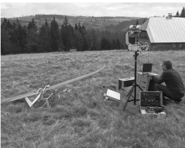
Fig. 1: Data acquisition at a test site in the Bavarian Forest National Park. Left: Preparing the UAV for its flight using a FPV flight guidance system. Right: UAV during its flight. Rough start and landing conditions as visible in the background can get avoided by using UAV platforms with hand launch and net landing capabilities as the shown power glider.
