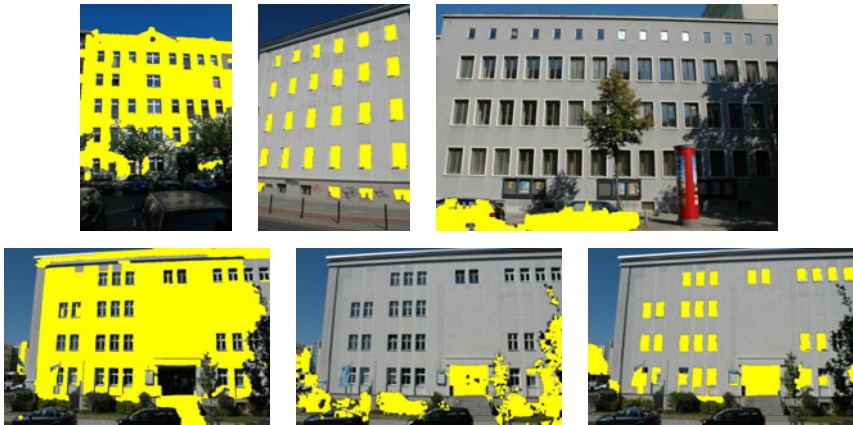
Fig. 3. Four scenes from Berlin (Germany) and classification results from the conditional Bayesian network. Top row: results w.r.t. classes building , window , and car , respectively. Bottom row: w.r.t. classes building , vegetation , and window , respectively.
