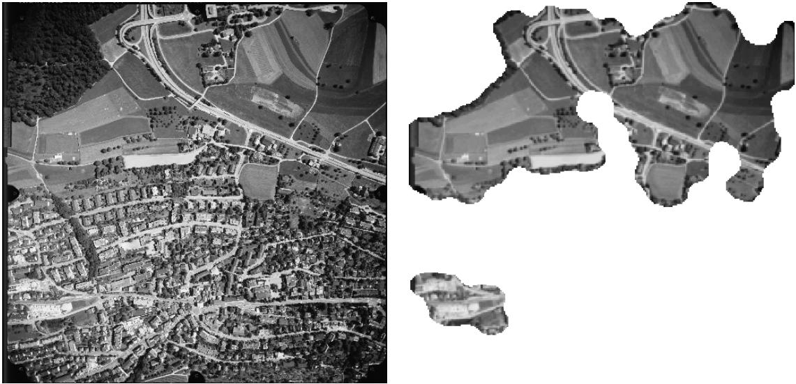
Figure 1. Left: Aerial image from the Zurich Hoengg dataset. Right: Texture based segmentation of *open rural area*.
