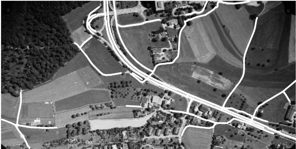
Figure 2. Result of road extraction for the upper part of Figure 1.
