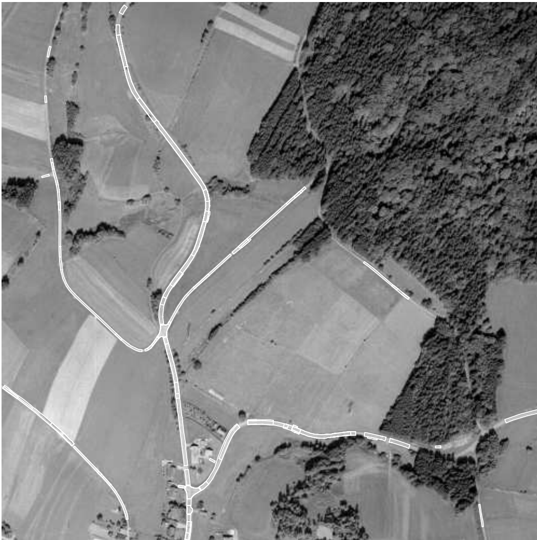
Fig. 5: Roads extracted in open_rural area (image size: 4000^2 pixels)
