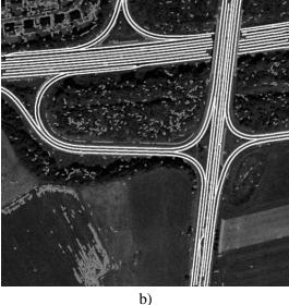
Fig. 6: a) Aerial image with extracted lines b) Selected road markings (white)
