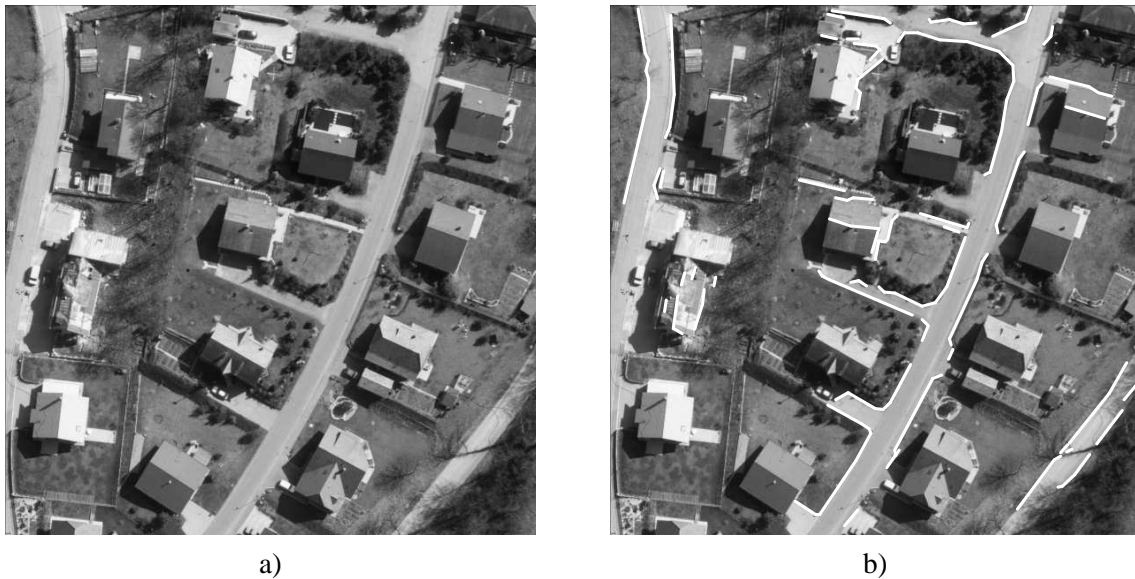
Fig. 8: a) Image 5897 of the Ascona testset b) Final result of the road extraction process
