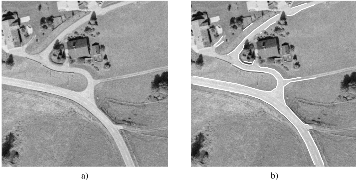
Fig. 7: a) Input image to the algorithm b) Final result of the road extraction process
