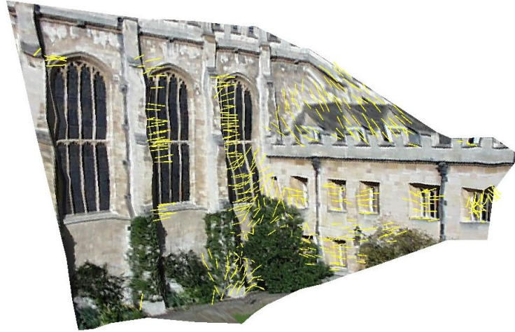
Figure 5.8: Positions and directions of 385 unknowns marked in yellow at pyramid level 0.
