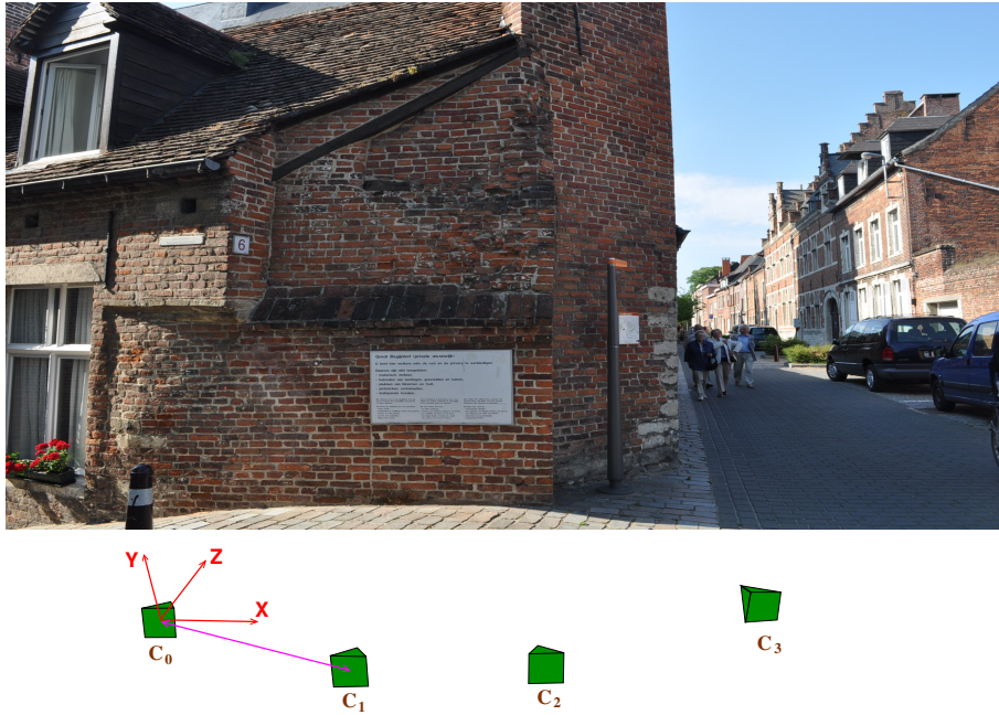
Figure 4.10: The position and orientation of the first camera C_0 supposed to define the origin and to point in the negative Z -direction together with the distance from C_0 to C_1 (scale) which is set to 1 are used to define the coordinate system.
