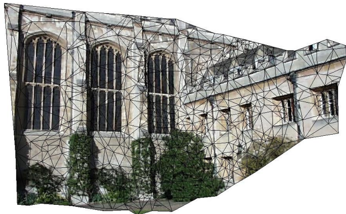
Figure 5.10: The final reconstructed 3D surface of Trinity corner.
