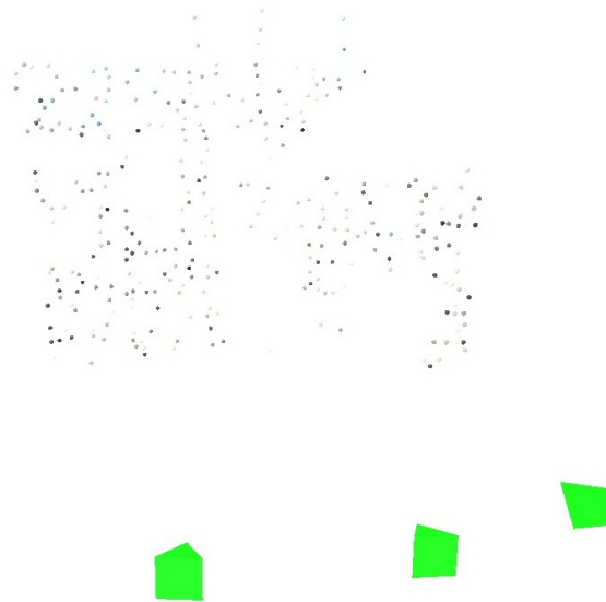
Figure 5.2: The three camera positions (green pyramids) and the 279 sparse 3D points.
