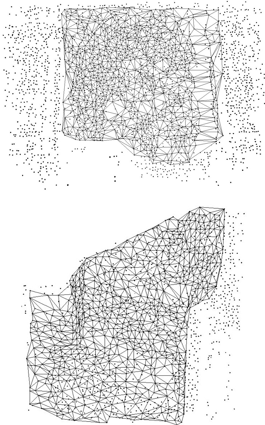
Figure 3.2: Wire-frame representation of a mesh (black lines) connected from predefined 3D points (black points).
