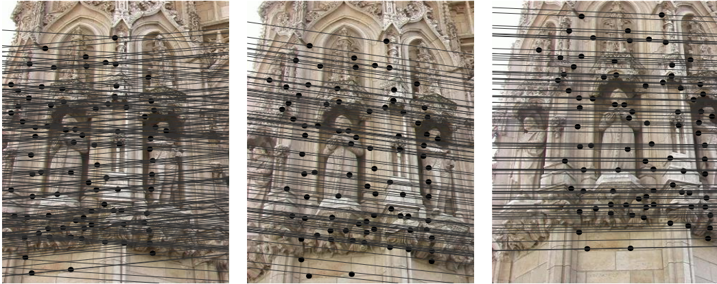
Figure 4.6: Wide baseline triplet with conjugate matched points and epipolar lines.
