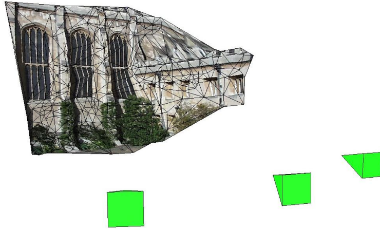
Figure 5.3: Triangulated mesh created from 223 points.
