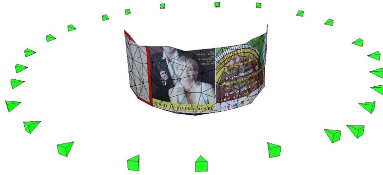
Figure 5.14: Triangulated mesh created from 63 points.
