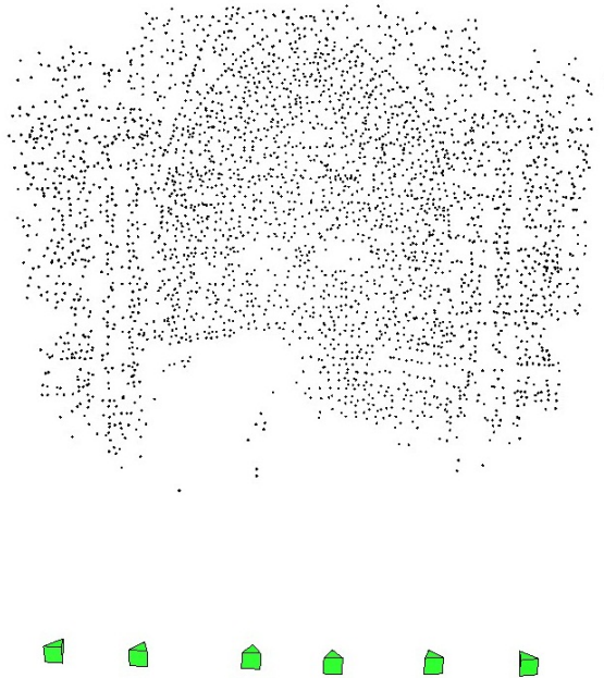
Figure 5.33: The six camera positions (green pyramids) and the 3286 sparse 3D points.
