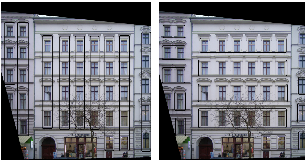
Figure 5.5: Window clustering. Left: Vertical clusters, windows are on the same column and have the same width. Right: Horizontal clusters, windows appear on the same row and have the same height.
