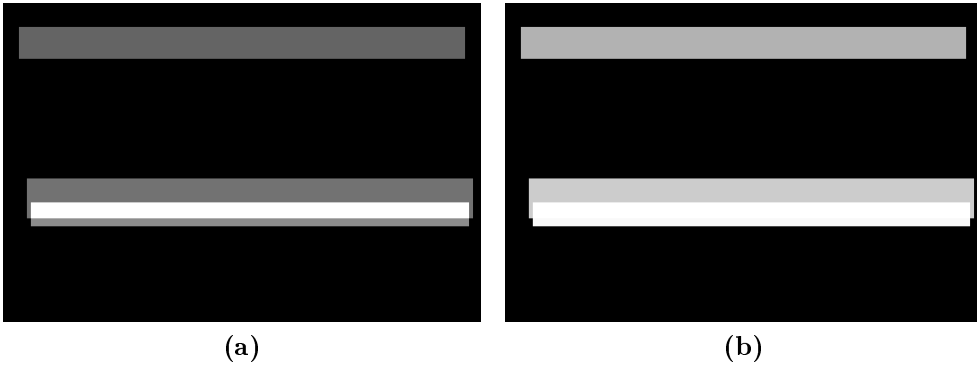
Figure 4.3: Effect of the normalization techniques. Suppose that there are three long balcony proposals, with probabilities (starting from the top) 0.7, 0.8, 0.98. The left image shows the min-max normalization used by other methods. Here, the upper region has a probability of less than 0.4, i.e., it becomes a region with low probability. The right image depicts our proposed normalization method. None of the regions obtains a low probability
