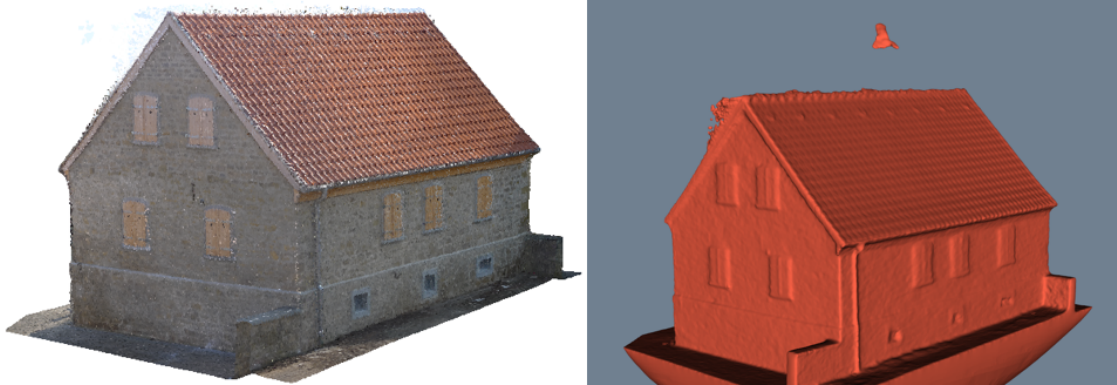
Figure 3.1: Automatic model creation from point clouds using classical meshing algorithms has been widely employed for small objects in indoor scenes. In this example, we applied Poisson reconstruction to point clouds from an SfM/MVS pipeline. The point cloud was manually filtered and everything but the immediate surrounding (left) cut-off. Besides lack of semantic information, the reconstructed triangular meshes (right) over-fit the scene capturing all fine details.
