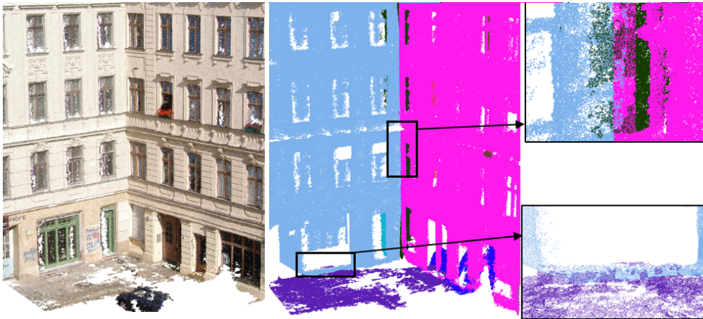
Figure 6.3: Results of segmentation overlapping at segment boundaries. 3D points at regions overlapping are assigned multiple labels. In this example, inliers on the lines of intersection of the two facades, as well as of the facades and the ground have multiple labels.
