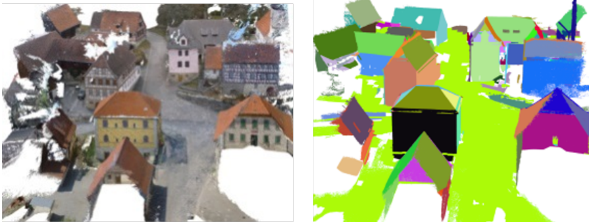
Figure 5.1: Building walls, roof elements, and the non-planar ground (right) segmented by our algorithm in a point cloud (left: 46 million points) derived from images by Structure from Motion/Multiview Stereo (SfM/MVS). The problem is formulated as probabilistic inference that robustly segments all patches in the scene.
