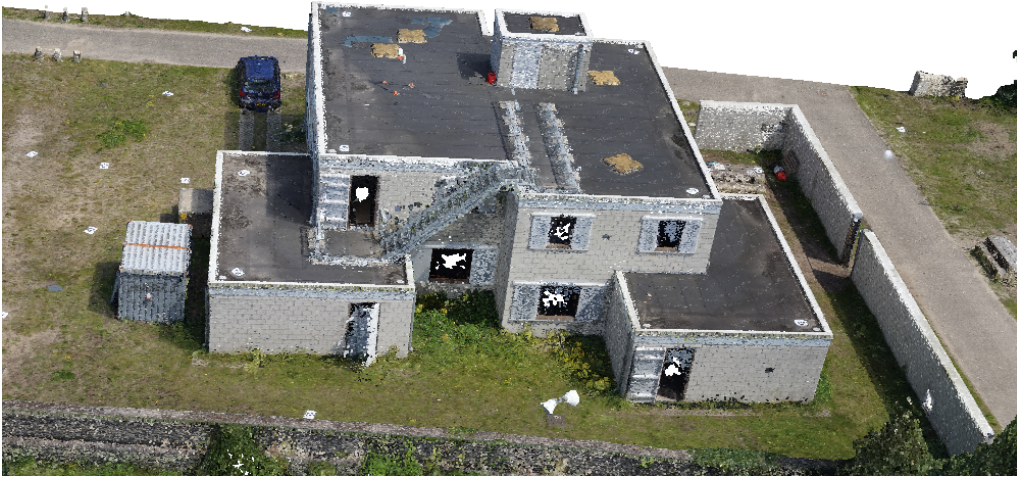
Figure 8.3: Point cloud derived from images by SfM/MVS. Besides reconstruction artefacts and noise, this scene has three major orientations: Two orientations for the walls and one for the ground together with the flat roof, making it particularly suitable for assessing the effects of changing parameters for clustering.
