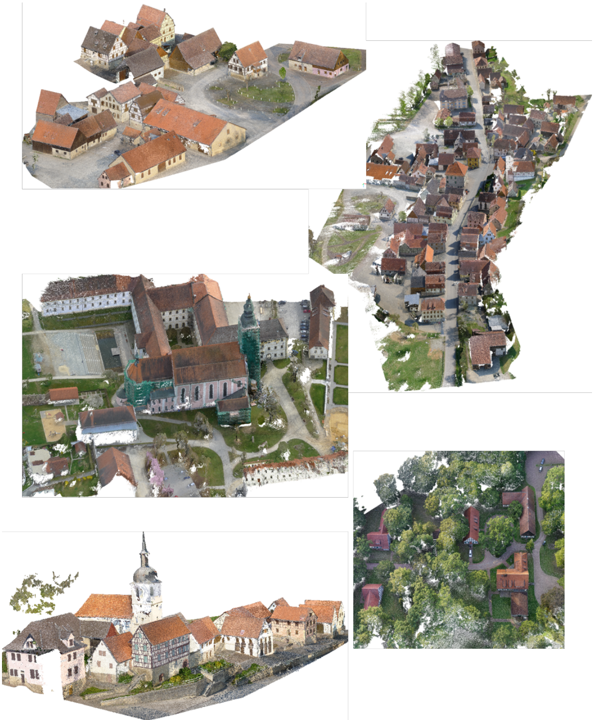
Figure 8.2: Examples of point cloud data from our test set. This data is derived from images via SfM/MVS. It ranges from 3D point clouds of single buildings to an urban block of 51 buildings captured with images of handheld cameras combined with images from UAVs.
