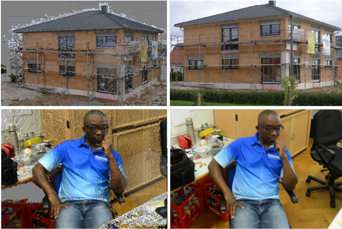
Figure 2.1: 3D point clouds produced from images by SfM/MVS are becoming very popular. These examples show two point clouds derived from a SfM/MVS pipeline for both an outdoor (top left), and an indoor (bottom left) scene. In both cases, each 3D point is associated with a corresponding color value r, g, b . This allows for a visual comparison with a 2D image (right) from the image sequence.
