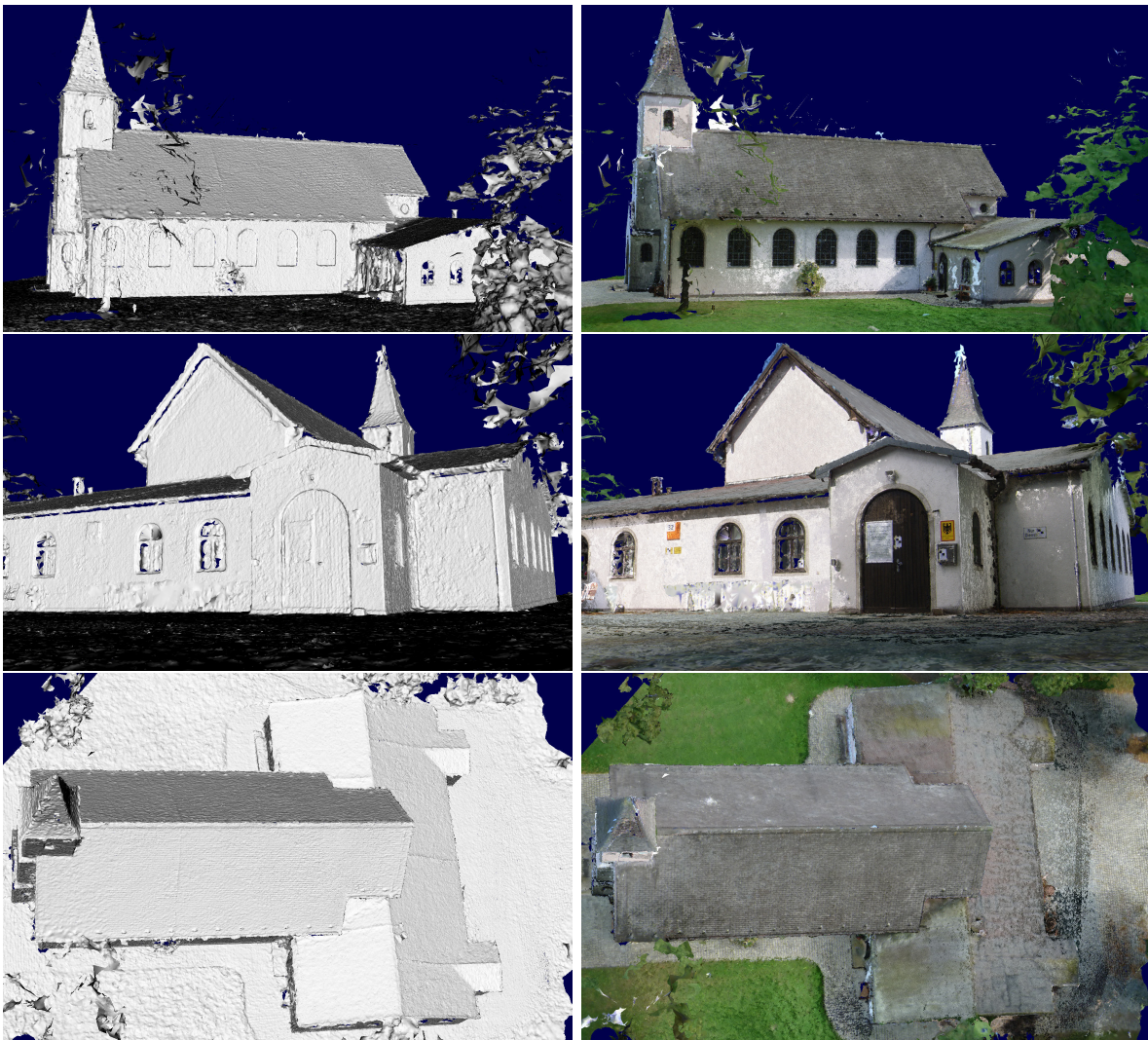
Figure 7.8.: Shaded and textured parts of the 3D surface model obtained from the image set shown in Fig. 7.7. The surfaces were obtained from 10 MP images taken from the air and on the ground. Moving objects such as vegetation were only partly reconstructed.
