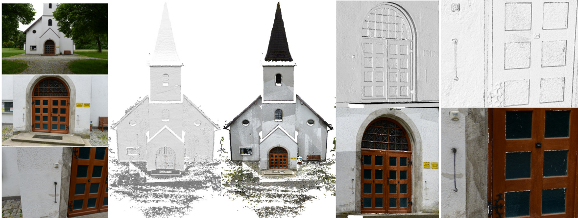
Figure 7.10.: Textured and shaded 3D model reconstructed from 54 images (left column). The images were captured at varying distances to the object. The multi-resolution method retains only the best qualities during the 3D surface reconstruction. The largest voxel is about 200 times larger than the smallest.
