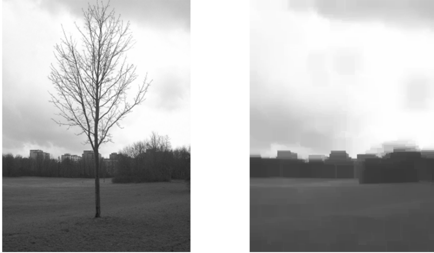
Figure 5.3: Background estimation: original image (left) and after gray-scale Closing (right).
