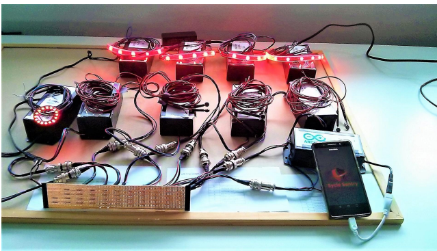
Figure 3. Visual, tactile and audible output modalities and a custom-built I2C-BUS constitute the Bicycle Exploratory Prototyping Toolkit for rapid exploratory prototyping.
