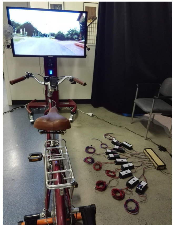
Figure 1. Workshop setup to develop an on-bicycle UI in close cooperation with the target group utilizing an Exploratory Prototyping Tool (right) for rapid hands-on prototyping in a collaborative environment.
