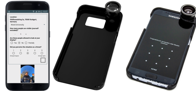
Figure 2: The rating app (left), the smartphone enclosure with fish-eye lens design (center), and the produced prototype (right).
