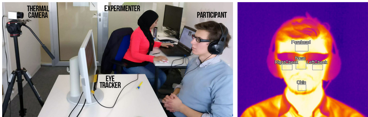
Fig. 2. Left: Experimental setup consisting of thermal camera and eye tracker facing the participant. Right: The facial features being monitored by the thermal camera (forehead, nose, left cheek, right cheek and chin).
