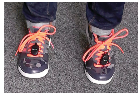
Figure 3. RunScribe is a pair of sensors that attach to the runner's feet in order to gather detailed gait data.
