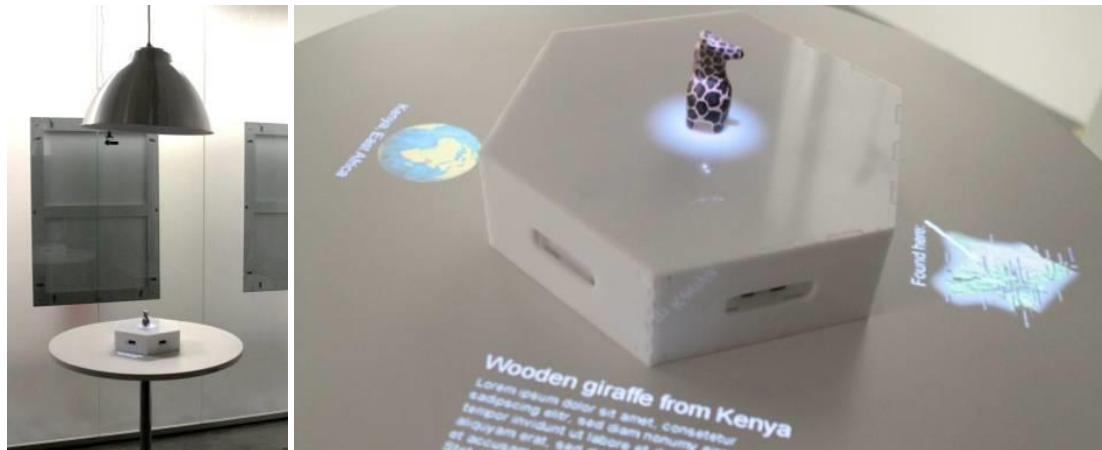
Figure 1: Plinth prototype designed in a participatory design workshop with cultural heritage professionals that senses visitors around an exhibit and projects content according their position
